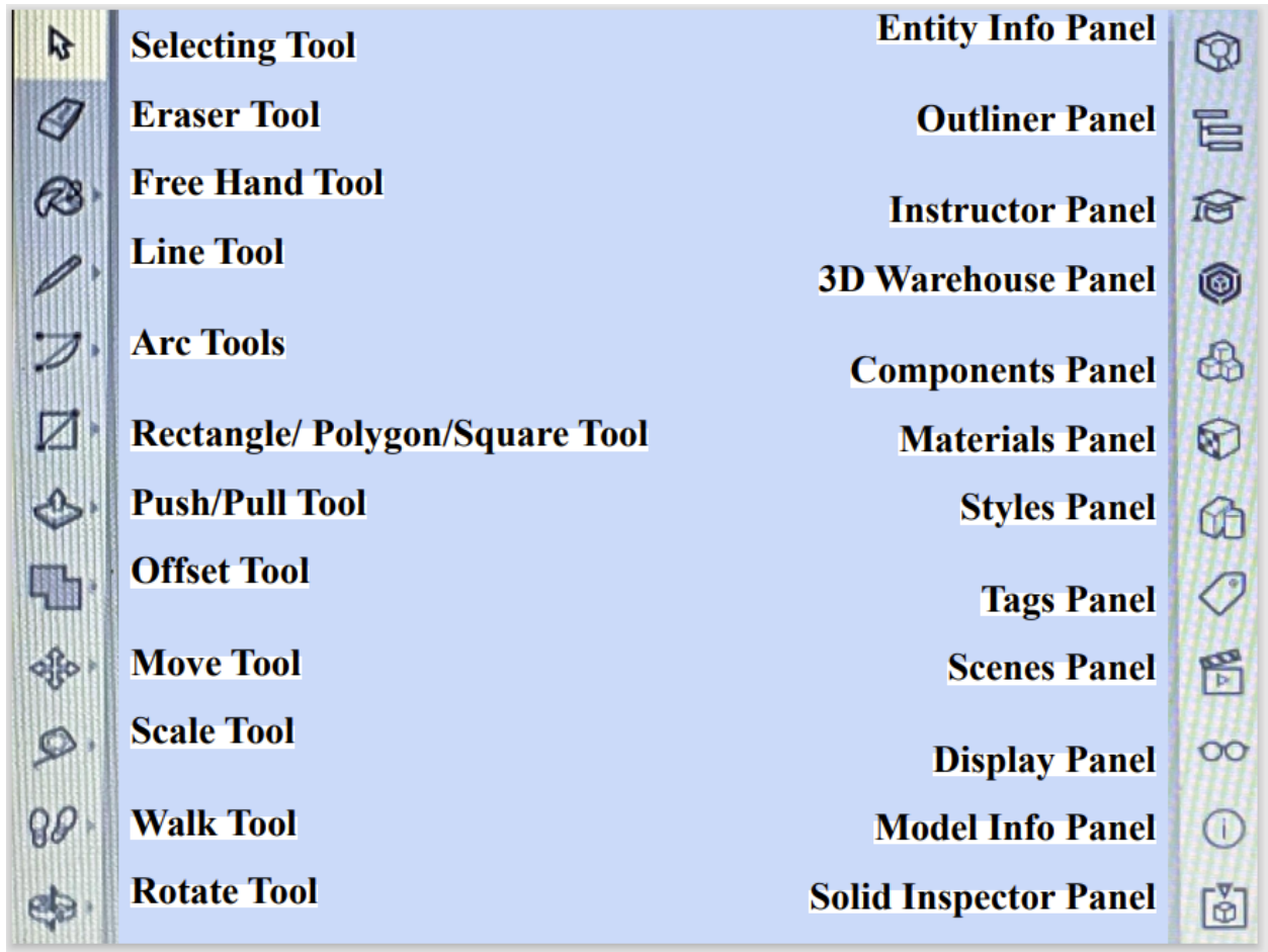
Fig. 1 SketchUp Tolls and Panels Identified
